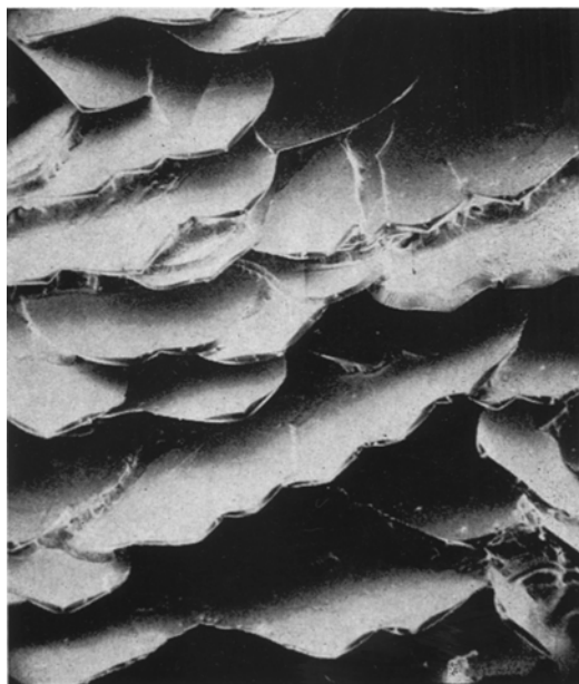
Figure 10 Scanning electron image of the lamella obtained by solidification of interdendritic liquid during decantation. ( \times 100 ).
