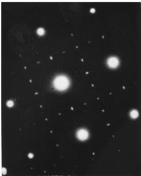
Figure 6 Diffraction pattern of selected area of Fig. 5 showing matrix and three precipitate reflections.
