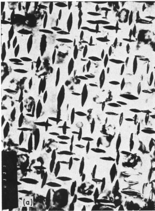
Figure 5 Transmission electron micrographs of a thin foil of alloy 12. (a) Bright field ( \times 46\,000 ), (b) dark field ( \times 46\,000 ).
